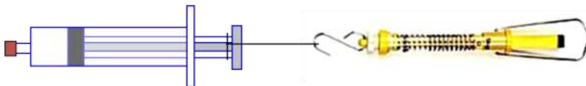
An empty syringe is blocked at the opening and the piston is attached to a newton balance, which is pulled.
