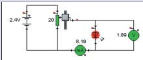
**Fig 1: Alternative layout and equipment for V vs I.**
