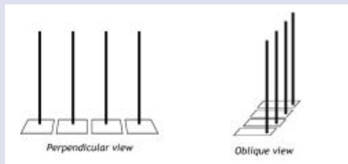
A festoon lamp can be mounted above one edge of a record. Then look towards the reflection of the lamp in edge of the record nearest to you.
