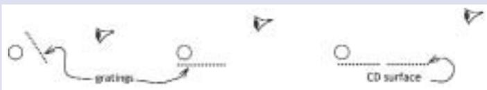
Side views showing methods of observing transmitted and reflected diffraction, and comparison with a CD
